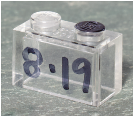
The 1x2 brick with no underside bar prior to bleach bath. Writing on side is one-pass, ink on stud is multiple coats.
