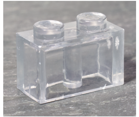
48 hours: Black on stud completely gone. Plastic remains clear and hard.
