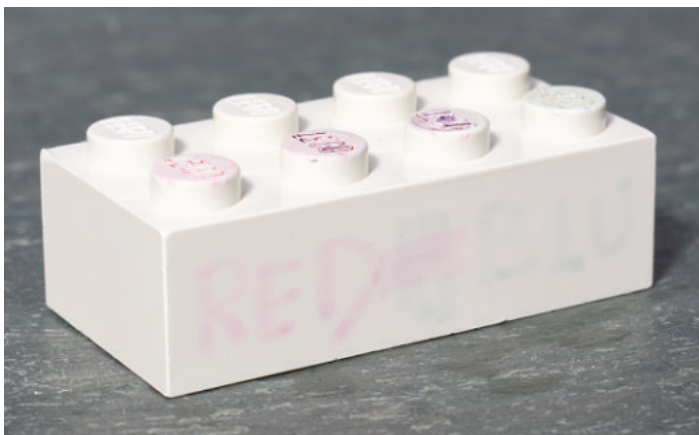
Day 4: fading continues, more evident on the studs.
