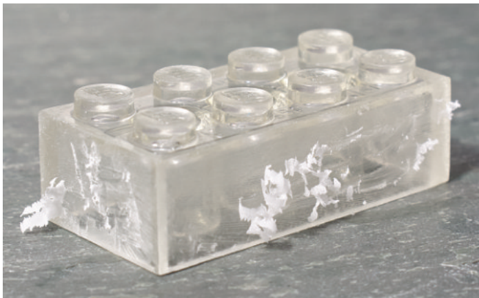
48 hours: Sharpie marks are completely gone, and as with the 2x2 brick the sides have gone cloudy and can be easily scuffed with a fingernail.
